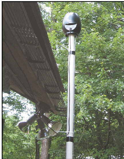
Figure 3—The Ultimeter Pro Rain Gauge must be in the open, away from overhanging trees and clear of the house or other structures that might block blowing rain.
